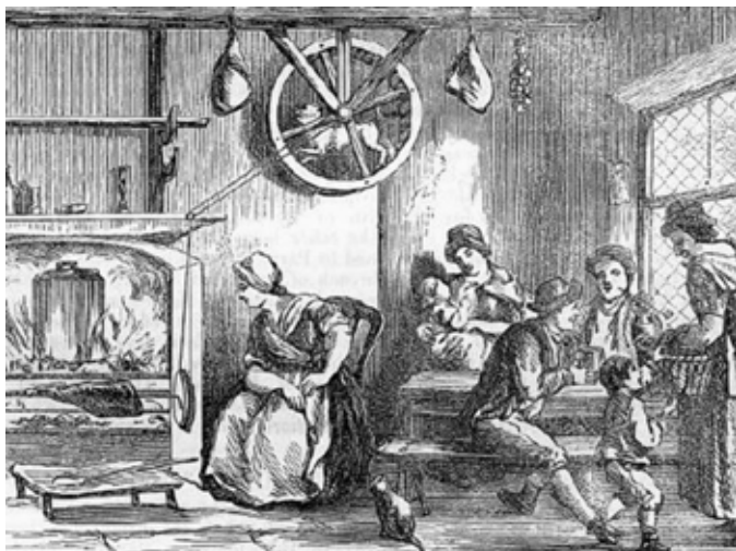
A turnspit dog in a wooden cooking wheel circa 1860. Engraving reproduced in Robert Chambers’ Book of Days .
